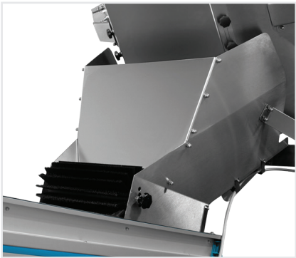
Dosing hopper between Bin tipper and Conveyor
